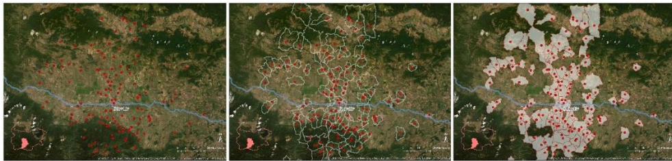
Fig. 2. Spatial join of waqf point data with village land polygons. Created by G. Boykov (2020)
